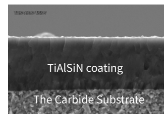
SEM Photograph of Coating
